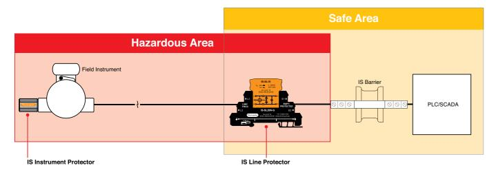
For complete technical specifications or to view the certificate of conformity for the Novaris intrinsically safe range of surge protection devices please visit **www.novaris.com.au**.
